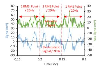
*Fig. 2. Signal and absolute signal as a function of time. RMS is calculated by taking the average deviation of the electrostatic data every 20Hz / 0.15sec time window.*
