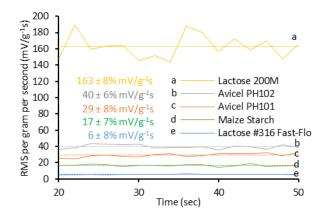
**Fig. 3.** RMS normalised against dw/dt as a function of time within a 30s time window. Mean mVS/g<sup>-1</sup>s for a material is indicated by dashed line and value of the same colour.
