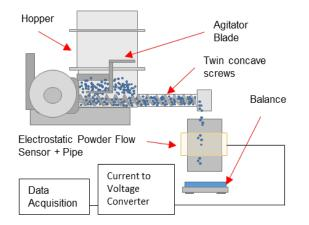
*Fig.* 1. *Experimental setup of volumetric twin-screw feeder, EPF and data measurement system.*
