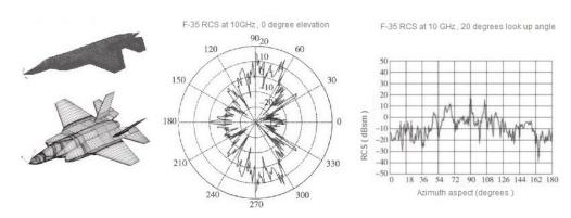
Note: software is treating the entire aircraft and all of its parts as purely reflective metal surfaces, addition of radar absorbing material (RAM) would further reduce aircraft RCS; Also effect of radar absorbing structures (RAS) wasnot simulated due to lack of data
