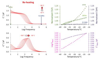
**Fig. 1** (LEFT) Real and imaginary capacitance spectra; (RIGHT) Extracted parameters: TOP real part capacitance C' at selected frequencies, BOTTOM peak frequency ( $F_{peak}$ ) and peak amplitude (C"peak)
