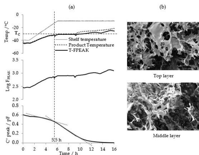
**Fig. 1.** (a) The temperature and TVIS parameter profile of 5% w/v lactose solution during the primary drying stage (b) SEM of top and middle layer of lactose cake at the end of the cycle.
