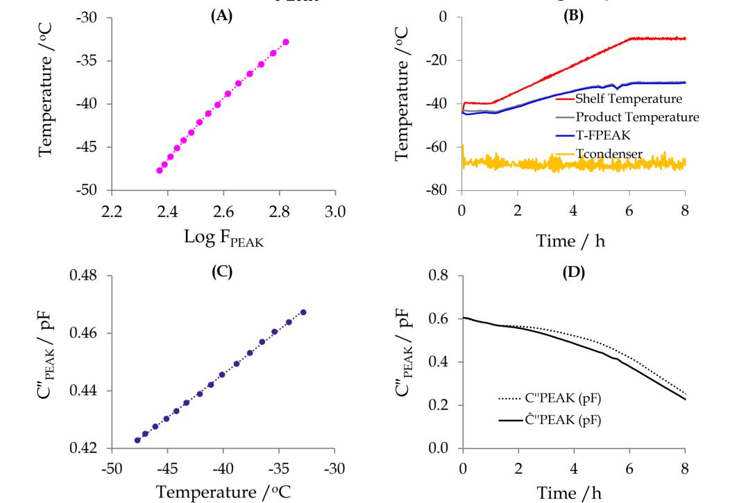
**Fig. 2.** The temperature and TVIS parameters profile of 5%w/v lactose solution during the primary drying stage. (A) Temperature calibration from re-heating step, (B) a predictive temperature during primary drying, (C)  $C_{PEAK}^{"}$  calibration from re-heating step and (D) Temperature-compensated  $C_{PEAK}^{"}$  ( $\hat{C}_{PEAK}^{"}$ )
